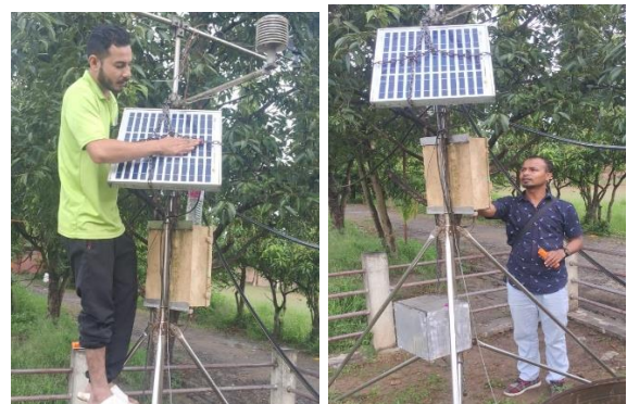
Installation of Automatic Weather Station
